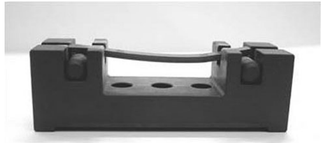
Fig. 1 The SiC flexure device and a tested (1500 °C) parallelepiped-shaped specimen
